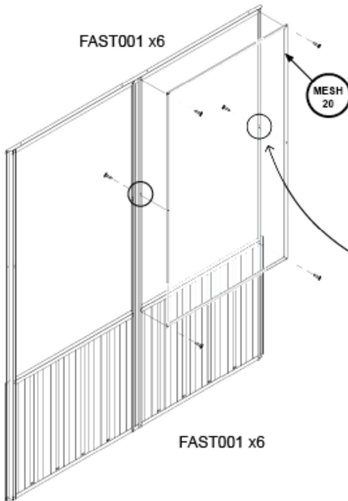
The mesh panels are fixed to the inside of the wall panels.
