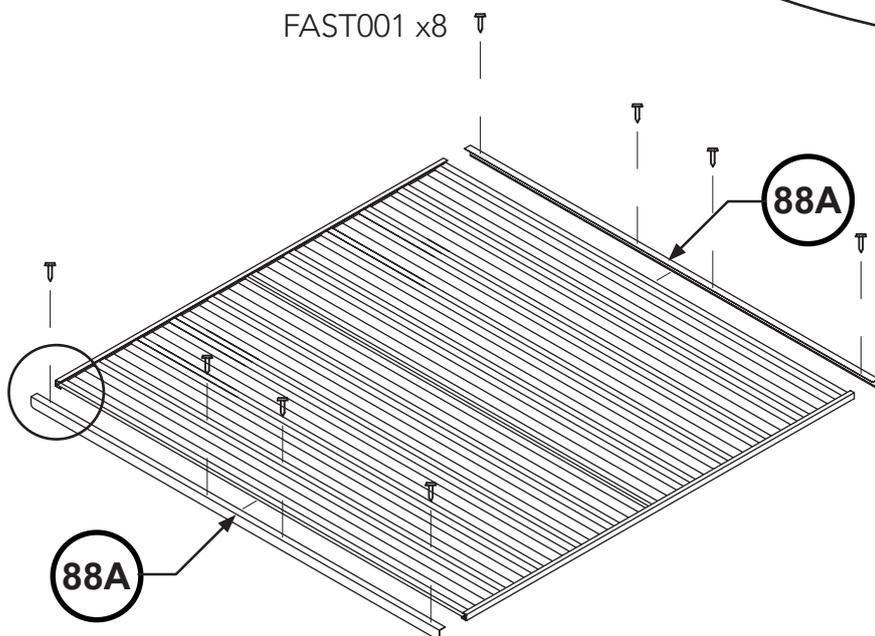
**3.** Attach the top and bottom channels using the SNAP-TiTE method.
