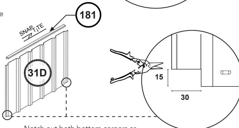
Notch out both bottom corners as shown using tinsnips.
