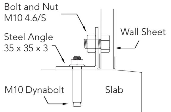
Each anchor consists of one nut, bolt, M10 dynabolt and steel angle.
