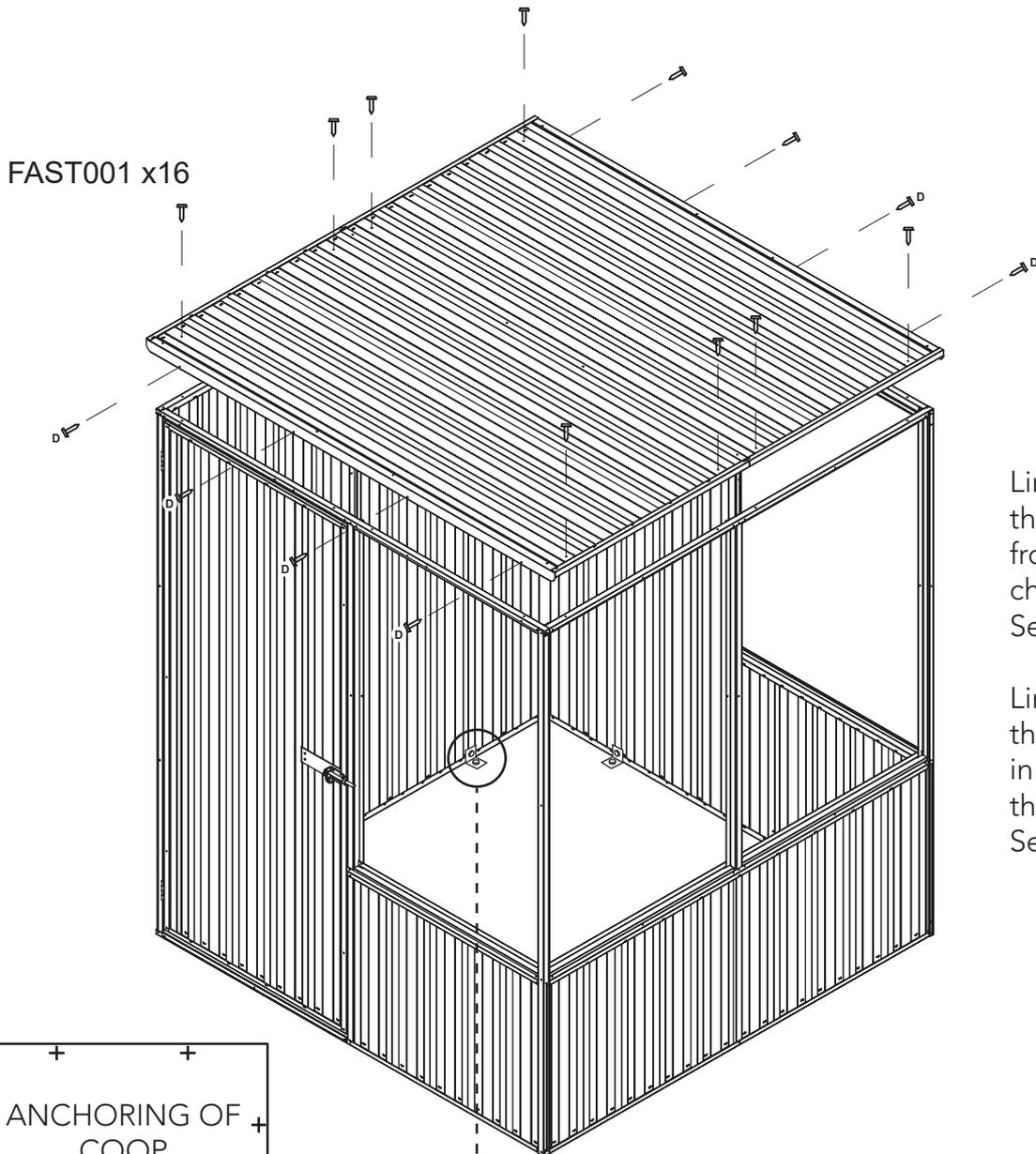
Line up the holes in the roof sheet with front and back top channels. Secure with screws.
