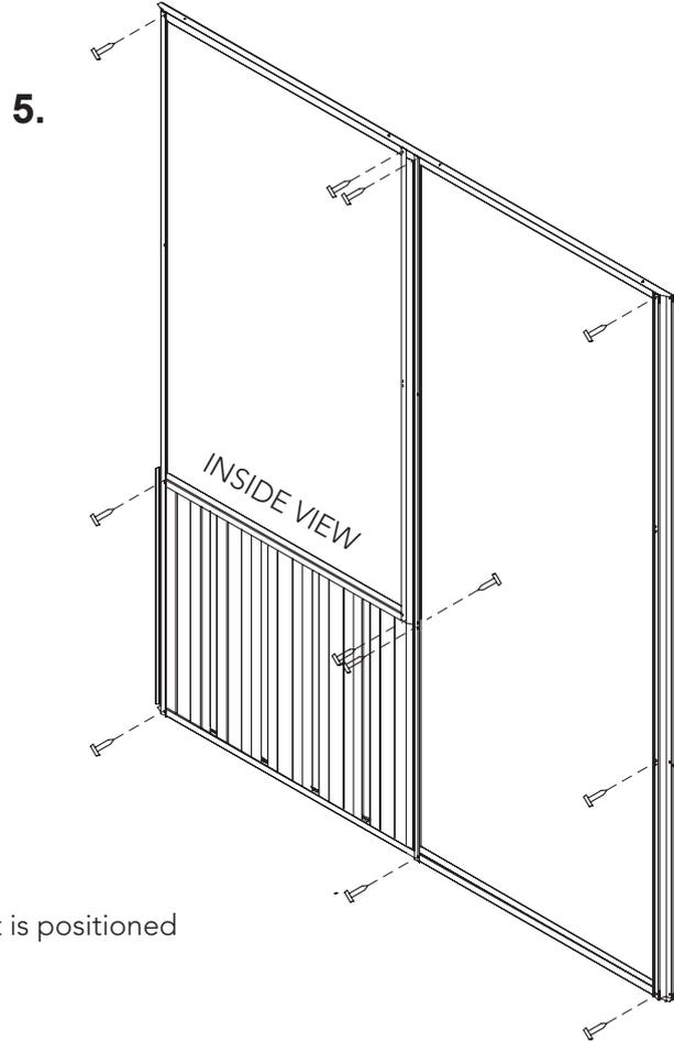
NOTE: 31D sheet is positioned behind jamb 89B
