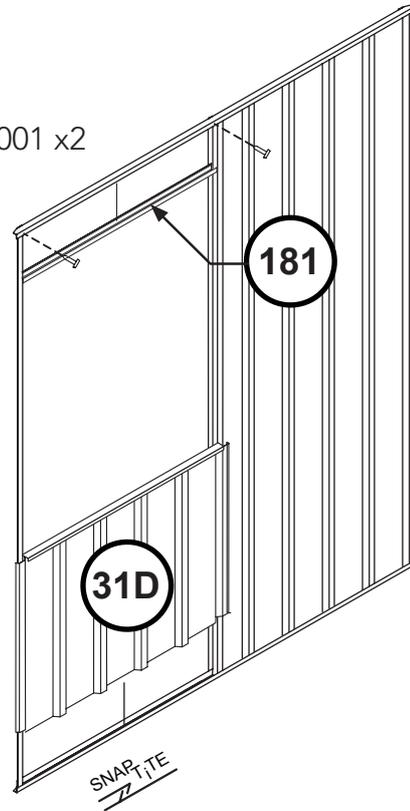
Notch out both bottom corners as shown using tinsnips.
