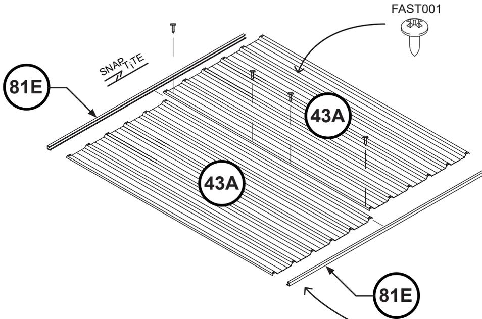
**1.** Overlap specified sheets as shown. Make sure ends are flush.
